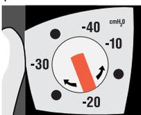
To lower regulator setting from a higher level (-40cmH<sub>2</sub>O) to a lower level (-20cmH<sub>2</sub>O), adjust regulator down to lower setting and then temporarily depress the manual high negativity vent located on top of the drain to reduce excess vacuum.
